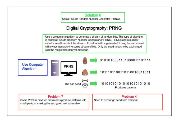
While PRNGs are deterministic and provide an easy way to get random numbers on a computer, they also introduced Problem 7, which is that most PRNG algorithms will produce numbers that start to follow a pattern. When the PRNG numbers used for encryption follow a pattern the result is just like repeating a text key with the Vigenère cipher, it makes it easy to crack the encrypted text.
