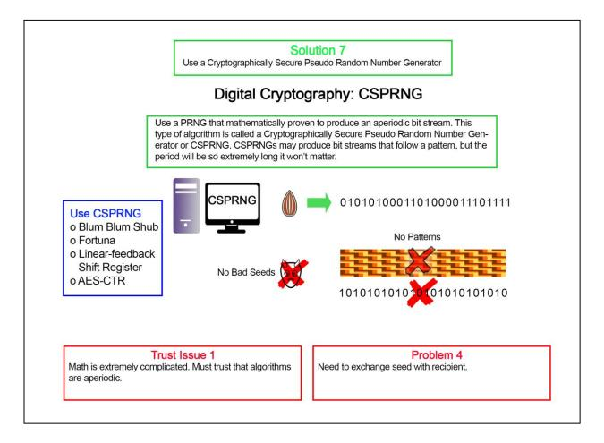
Tying this all together, modern encryption uses something similar to the Vigenère cipher called the Vernam cipher, which works on binary data instead of text characters. The Vernam cipher uses the XOR function instead of the tabula recta and uses bits generated by a CSPRNG as the key. The only information the message recipient needs to regenerate the key bits is the seed for the CSPRNG. Finding a way to securely exchange the seed for the CSPRNG is a problem that must be solved.
