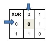
Or if the plain text bit is a 0 and the key bit is 1 the cipher text bit would be a 1 as shown in the following figure.
