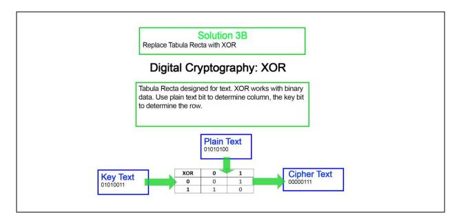
Using the Vernam cipher and the XOR table solved Problem 3, which brought us to finding a solution for Problem 4, which is generating a One Time Pad. In this case the OTP needs to be a string of random bits that can be XORed with the binary plain text data. The first step in this process was learning about true random numbers and true random number generators.
