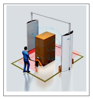
broadcast by a set of pillars like those you see at store entrances. The RFID pillars broadcast energy at a specific frequency which is enough to supply power to the RFID chip in tag, essentially waking it up and telling it to broadcast its ID information. The information from the RFID chip is read by the pillars, which decide how to handle it.
